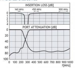
The DIPX 225/330 makes it possible to use only one antenna for the operation of two transceivers (one in each range). See the figure below. The antenna must be a dual-frequency antenna, e.i. it must be resonant on the actual frequencies in the two bands.
