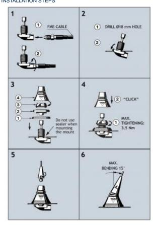
PLEASE NOTE: When tightening the revolving nut (see picture 4), special care must betaken to keep the spanner in the correct position.
